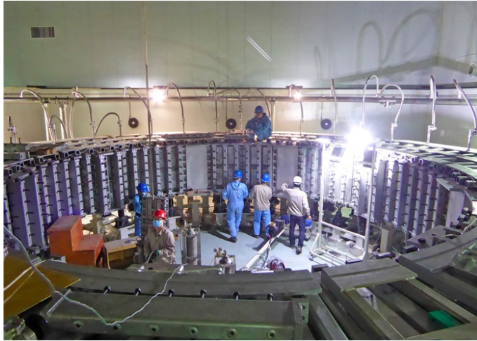
Technicians preparing for Vacuum Pressure Impregnation on PF6, ASIPP, Hefei, China
