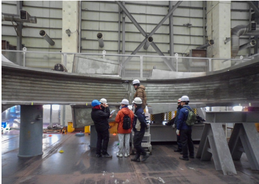
At Hyundai Heavy Industries in Ulsan, Korea, the outboard leg sub-assemblies were first fitted together to verify manufacturing precision
