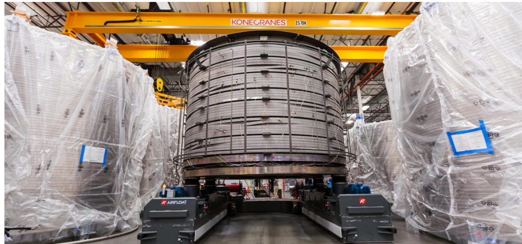
Transfer of central solenoid module coil to the heat treatment furnace
