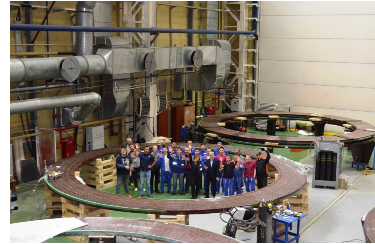
Completion of Vacuum Pressure Impregnation on 8 DP for PF1, Efremov, Russia
