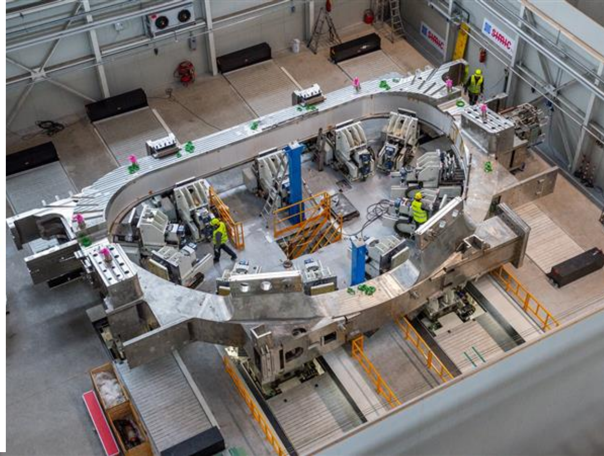
Europe's first Toroidal Field coil has been inserted in its case
