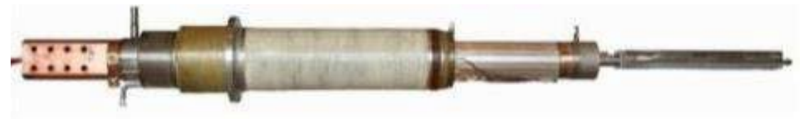
68 kA Trial Lead Developed by ASIPP
