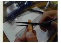
2. Bend it 90 degrees at 5 mm from both ends. Be careful not to apply too much stress on the middle 1 cm part, which is main part for magnetization.
