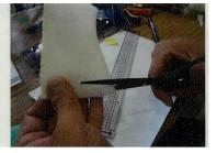
5. Put the sponge on the superconducting tape, then wrap it with aluminum tape. Make (Leave) a slit at the top surface of the wrapped rectangular piece for LN<sub>2</sub> infiltration.
