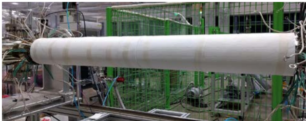
Covering thermal isolation (cerac paper, 5 mm, 3 rd layer)
