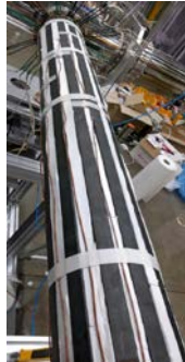
Inserting thermal Isolations (1 st layer, cerac paper)
