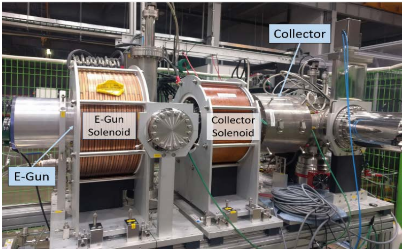
Figure II.18. (Upper) Cross-section view of e-gun/collector test bench: ① e-gun, ② gun coil, ③ gate valve, ④ collector coil, ⑤ vacuum breaker, ⑥ drift tube #11, ⑦ magnetic shield, ⑧ collector body, ⑨ repeller, ⑩ EBIS stand, (Bottom) Photograph of the installed e-gun/collector test bench.
