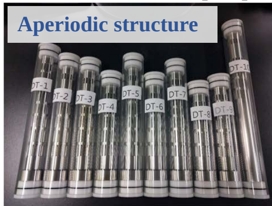
Vacuum-firing (1050 °C, 2 hours)
