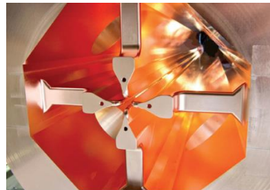
The Linac4 radio frequency quadrupole. image credit: M. Vretenar
