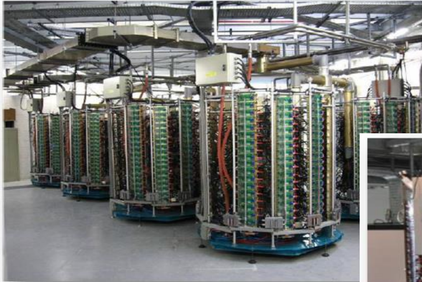
SOLEIL 45 kW @ 352 MHz tower solid state amplifiers (2004 & 2005)
