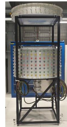
Figure 13: 2 MW 200 MHz CERN-SPS SSPA.
