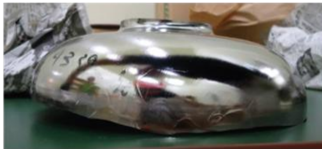
Half-cell made by large-grain disk
