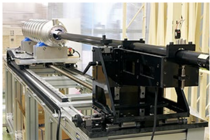
Inspection of inner surface
