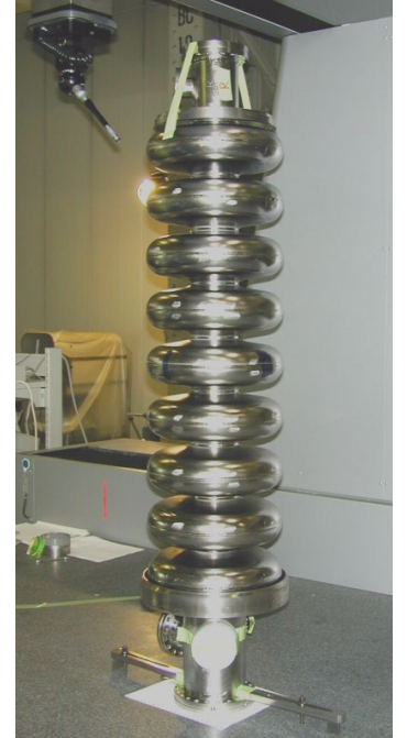
J-ADS 972MHz 9-cell Cavity ( \beta=0.73 )
