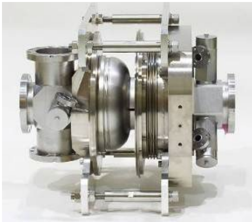
cERL Injector 1.3GHz 2-cell Cavity
