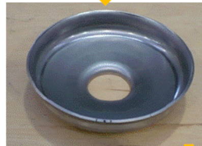
Half-cell No wrinkles, cracks
