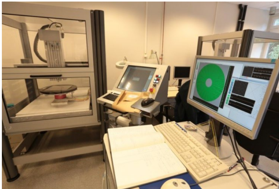
Eddy current scan of Nb sheet
