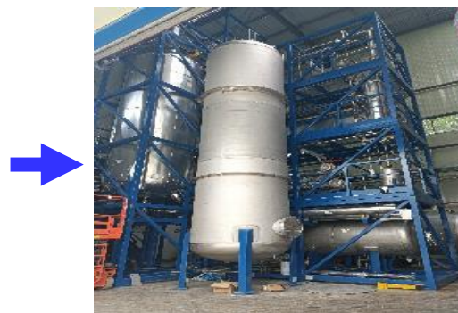
2) Distillation for radiopurity
