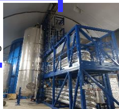
4) Gas stripping to remove Rn and O 2
