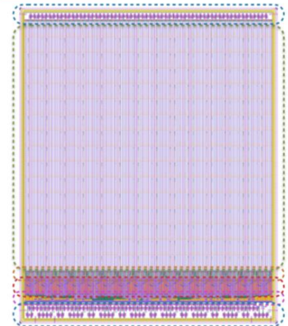
Arcadia by Italian groups for IDEA vertex detector LFoundry 110 nm CMOS
